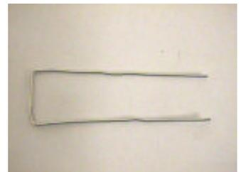
Bend the end of each leg in at 90 degrees as shown and clip each 'ear' back to about 2mm in length with the wire snips .
