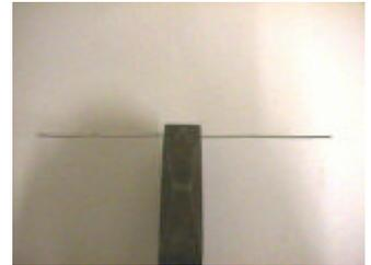
Bend down each leg at right angles to the plier jaws. Trim the legs with the wire snips so they are the same length.
